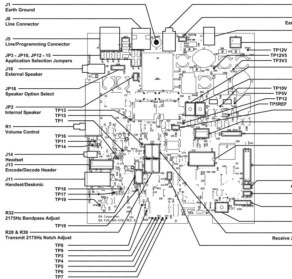
– J9 Foot Switch — JP1 Earth Ground Selection – J7 Wall Transformer — J2 **Alternate Power** - SW1 **Bootloader Mode** – SW2 **Test Mode** - JP16 **High Impedence** — J8 HUHS – JP15 **CPLD JTAG** — J10 **Keypad Interface** — J12 Test Header — JP17 **ATTiny Reset Enable** —— JP19 **PIC Reset Enable** — J4 **PIC JTAG** - SW3 Reset - R29 & R40 Receive 2175Hz Notch Adjust — JP11 MSK Baud
