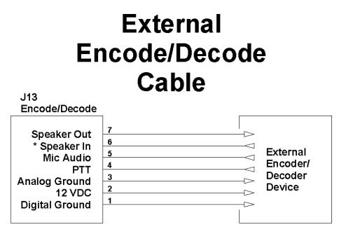
\* The removal of R19 is required for the proper use of the this signal.
