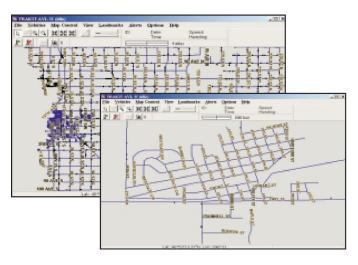
Real-time fleet tracking using maps from ESRI shape (Arcview) ormid/mif (Mapinifo) sources. Once in a WGS84 and geodedic lat/long format they become a full-function backdrop for TRAKIT vehicle monitoring. Installed in the base computer dispatchers can have complete and up-to-the-second information on the location and status of any vehicles in the fleet.
